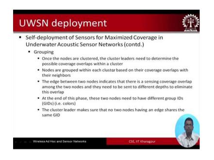
So, once these nodes are clustered the clustered leaders need to determine the possible coverage overlaps within a cluster. So, these nodes are grouped within each cluster, based on the coverage overlaps with their neighbors. The edge between the 2 nodes indicates that there is a sensing coverage overlap among the 2 nodes and they need to be
