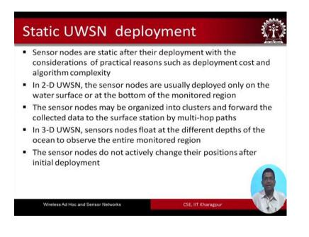
So, in static deployment the sensor nodes are static after their deployment with the considerations of the practical reasons such as the deployment cost and algorithm complexity. So, as the name suggests over here again. So, these sensor nodes somehow you make them static either you make them static on the ocean surface you know just you know just below the ocean surface you tag them through some buoys or something like that or you tag them in such a way that they are not going to move right.
