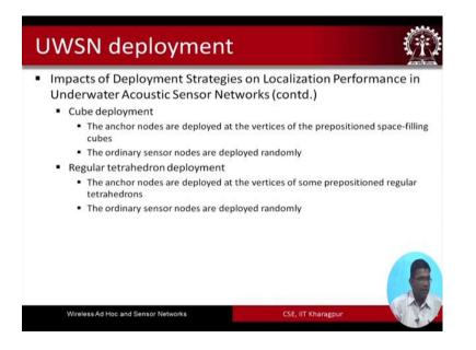
In a cube like deployment the sensor nodes are deployed at the vertices of the prepositioned space filling cubes the ordinary sensor nodes are deployed randomly around those and in the regular tetrahedron deployment the anchor nodes are deployed at the vertices of some prepositions regular tetrahedrons and the original ordinary sensor nodes are deployed randomly around them.
