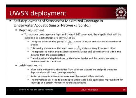
So, there are other phases after the clustering and grouping phase, there is a depth adjustment phase. So, to improve the coverage overlaps and the overall 3D coverage. The depths that will be assigned to each group are computed using this particular formula. So, the space between 2 groups is should be maintained as D by G plus one where D is the depth of water and G is the number of groups. So, this spacing makes sure that each layer is G by sorry D by G plus one distance away from each other.
