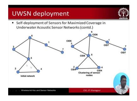
So, this is the initial network and from this you are going to form different cluster IDs like this right. So, these are the different cluster IDs and from these cluster IDs one can get the this is this is the cluster head right. So one can calculate the cluster head.
