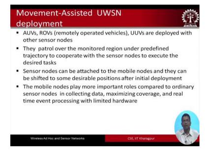
So, in movement assisted underwater sensor networks AUVs and ROVs etcetera are also deployed with other sensor nodes. So, these AUVs and ROVs etcetera UUVs they basically patrol over the monitored region, under predefined trajectory to cooperate with the sensor nodes to execute the desired tasks. So, the sensor nodes are deployed at different places and these AUVs ROVs etcetera they are going to move around these sensor nodes.
