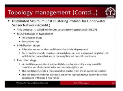
So, this protocol is called minimum cost clustering protocol MCCP which consists of 2 phases the first phase is the initialization phase. The next one is the execution phase in the initialization phase basically as this name suggesting in initial it talks about initial deployment of the different nodes and each candidate node basically after deployment it constructs the neighbour set and the uncovered neighbour set which is the nodes that are in the neighbour set, but still our candidates.
