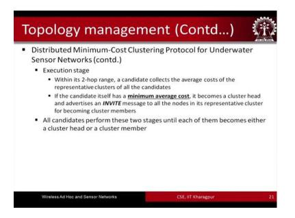
In the execution stage when it is 2 hop range within its 2 hop range; that means, within the 2 hop range of a node a candidate collects the average costs of the representative clusters of all the candidates if the candidate itself has a minimum average cost it becomes the cluster head and advertises an invite message to all the nodes in its representative cluster and as for becoming the cluster members.
