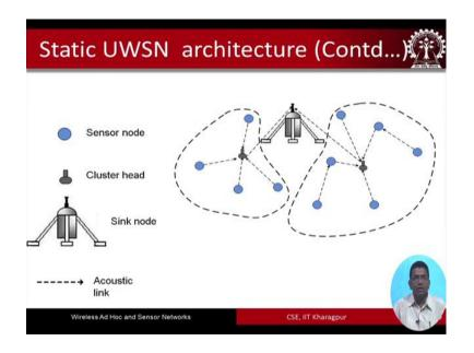
So, here is a picture of the static UWSN architecture here we have these blue coloured sensor nodes plus we have a cluster head to cluster heads are shown over here the 2 clusters and the corresponding cluster heads are shown and there is a sink node which basically connects with these cluster heads.
