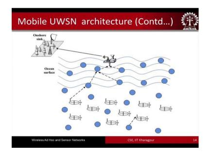
And here is a picture of the mobile sensor networks mobile underwater sensor networks. So, you can as you can see that you have these different sensor nodes which are not anchored like in the previous case, but these are like you know floating in the underwater column and also there are some UAVs which are also floating along with them.
