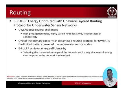
So, I am not go gone through it, but each of these 2 phases they talk about you know how to perform medium access control in these environments in an energy efficient manner routing is a very important problem in any network and similarly for underwater sensor networks as well. So, one of the primary concerns in designing a routing proto protocol for these networks is the limited battery power of the sensor nodes.
