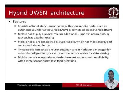
So, then we have the hybrid underwater sensor network architecture which consists of a lot of static sensor nodes with some mobile nodes and these mobile nodes are typically the AUVs and ROVs the mobile nodes basically play a pivotal role for additional support
