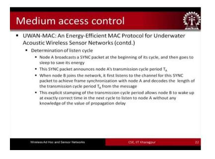
So, a MAC protocol was there are different MAC protocols that have been designed one MAC protocol is the UWAN MAC which is the full form is an energy efficient MAC protocol for underwater acoustic sensor networks. So, here basically it works in different phases the determination of listen cycle determination of transmit timers and so on.
