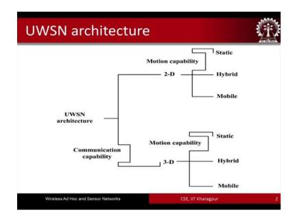
So, when we talk about architecture the underwater sensor network architectures that have been proposed they can be classified into 2D architecture and 3D architecture. So, under 2D depending on the motion capability or the motion of the different nodes in the network they can be even further classified into static 2D, hybrid 2D or mobile 2D, similarly for 3D as well static 3D, hybrid 3D and mobile 3D architectures.
