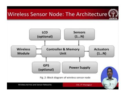
So, here is the overall architecture of a wireless sensor node. So, little later on during this lecture I am going to present to you a wireless sensor node that we have developed
