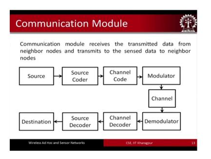
So, that is the memory unit and then you have the communication unit. So, for communication basically the data is received from the source node and then once it is received you know it goes through the source coder, then the channel coding is performed modulation is performed goes to the channel you know at the destination and it is demodulated and then general decoding is performed source decoding is performed and the data is finally, delivered to the destination module destination node.
