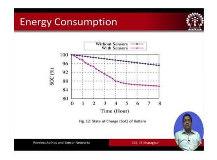
Changing the firmware of the node. So, just by changing the firmware of the node this node you know as a whole can be used for something different applications. So, these are the state of charge in the battery using this one node. So, you no need to explain we can without sensors how the charge you know degrades over time is shown in this particular plot.
