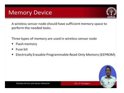
So, this is about the controllers then we have the memory device, the memory device which basically will store the data right. So these data have to be stored in the memory space. So, this device basically store state and there are different types of memory devices that can be used flash memory could be used fused bit memory could be used EEPROM based memories could be used.
