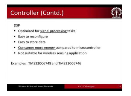
DSP based controllers are also there these are particularly attractive where signal processing tasks are quite heavy and; however, you know DSP based controllers they basically consume more energy compared to the microcontrollers.
