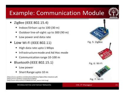
So, these are some examples of different communication modules that could be used in a sensor node. A ZigBee based communication could be used which is quite popular. In fact, ZigBee is popular for use in sensor nodes ah
