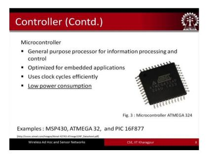
So, here where the picture that we see is that of a microcontroller called at mega 3 to 4 and this is a microcontroller which basically consumes very low power and uses the clock cycles very efficiently, and this is very attractive for use in embedded applications in general and ah.
