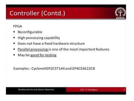
And sensor nodes in particular FPGA based controllers are also attractive particularly for parallel processing applications then.
