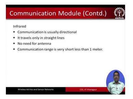
Infinity it is also very popular you know it is a communication that is directional in nature; that means, that it is travels in straight lines there is no need for antenna and the communication range is very short very short means less than a meter or so.
