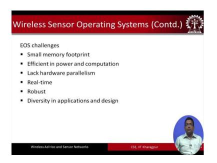
Like wireless sensor nodes and these embedded wireless sensor devices they have small memory footprint they are efficient in power as well as computation power consumption. And computation there you know basically support typical embedded applications are real time in nature. So, they support to real time applications they are robust and they support divers different types of applications with and become in in different types of designs.
