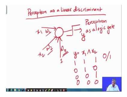
And it can be it was originally used to use Perceptron as a logic gate logic; logic gate, let us see how to do that suppose I have 2 inputs 2 weights and there is a bias term w naught and there is a threshold activation function.
