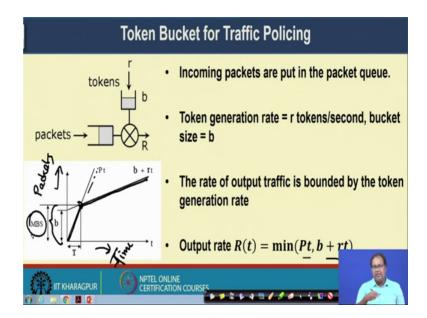
We will go for another algorithm for traffic policing and shaping it is called a token bucket algorithm. So, the token bucket algorithm the idea is little interesting and it support something called traffic burst.
