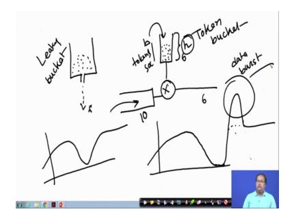
So, in case of leaky bucket what was happening, you had this leaky bucket and a small hole in this leaky bucket. So, whatever packet you are getting here you are taking it output at a constant rate. Now in that case if there is a no at a constant rate r in that case if there is no packet then there would be no output.
