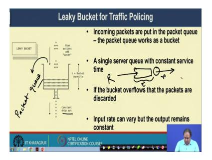
So, the first mechanism that we are going to talk about is leaky bucket algorithm. So, although in the slides I have mentioned that leaky bucket for traffic policing, but as I have mentioned the ultimate mechanism is a combination of traffic policing and traffic shaping. So, this leaky bucket mechanism by idea it is very simple, the idea is that you have a bucket just what you are seeing in the example.
