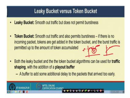
So, here is the difference between the leaky bucket for this is token bucket algorithm. So, the leaky bucket algorithm it smooth out traffic, but it does not does not permit
