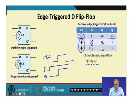
Now, let us talk about the edge triggered version of a D flip flop; it is exactly similar to an S R flip flop. First this symbolic notation exactly same; so I can show it either positive edge triggered like this negative edge triggered like this. This is single input D, this state table also will look like this if the clock there is no leading edge positive edge triggered; no change if there is a clock edge.
