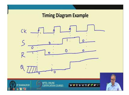
Suppose I have a clock signal let us say I have a clock let us consider there are 4 such pulses coming clock signal. And the flip flop is positive edge triggered I am assuming it is positive edge triggered, it is triggered on this edge this triggered on this edge.
