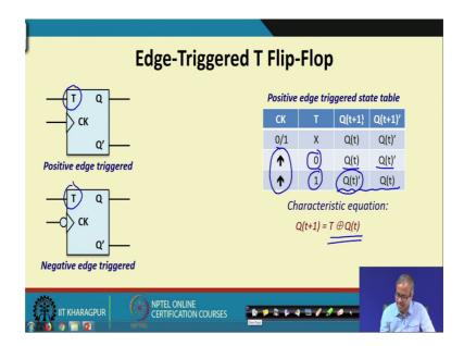
Now, there is another kind of a flip flop which you can say is a special case of a J K flip flop; this is called a toggle or a T flip flop. So, a T flip flop has a single input T as this diagram shows there is a single input T this S this is the positive edge portion negative edge portion and what this T flip flop says; if T is 0 there will be no change.
