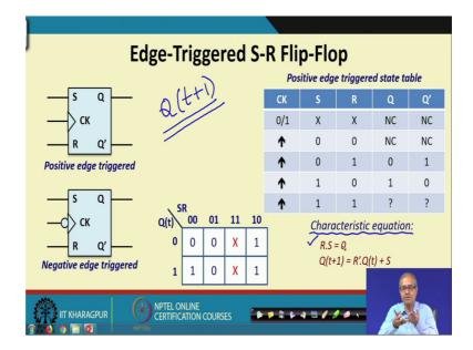
Let us now look at a edge triggered S-R flip flop; now you already know what an S R latch is let me try to explain what is shown in the slide. First is this symbolic notation in a diagram how you show and S R edge triggered flip flop. You see in an S R latch you have S and R Q Q bar outputs; here in addition you have another input called clock and this is how you show a clock just by a this angular symbol here.
