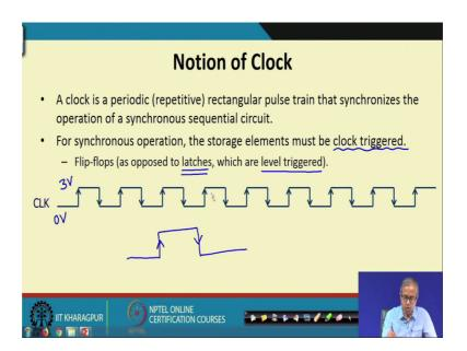
So, we shall be talking about clocks, the notion of a clock and how we can modify our design of the latch to make it a flip flop, which can be operated by a clock. Now let us try to understand why we need this kind of a clock and what is a clock?
