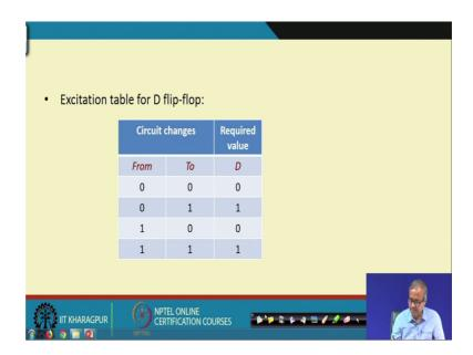
So, in a similar way we can construct the excitation table for the D flip flop; say for D flip flop if you want to change from 0 to 0, I have to apply 0 in the D input that 0 will go in; 0 to 1 I have to apply 1, 1 to 0 have to apply 0 1 to 1 I have to apply 1.
