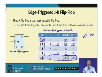
Now, let us talk about another kind of a flip flop called J-K flip flop. J-K is the most versatile of the flip flop versatile means it is more powerful than the other kind of flip
