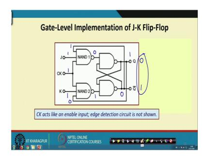
Now, let us look at the gate level implementations of a J K flip flop. Here I am just showing this diagram where we have referred to has here clock, but we have not shown any edge detection circuit we shall discuss it later, but assume that somehow some edge detection mechanism is there. So, when ever clock edge comes then only here some 1 comes.
