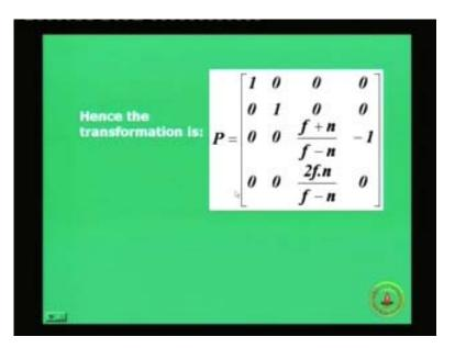
This is the transformation matrix. Now this transformation matrix will handle the z transformation from the finite view parameter to a canonical view volume. What about u and v with respect to x and y, well we also have to go to any one of these axis and the u v axis transformations of the pyramid are understood by taking the side view again.
