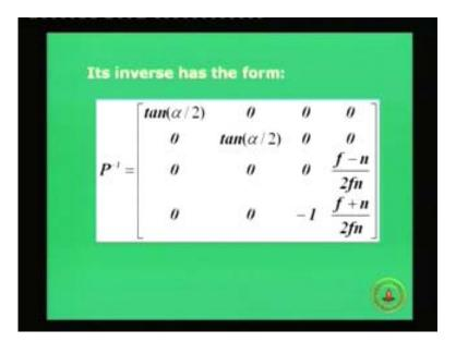
You can try out the inverse of p which should be this. You can note it down for the time being and practice at home, 4/4 matrix not a very difficult one. This is the matrix p and this is the inverse of the matrix which is given as cot alpha becomes tan alpha by 2. Diagonal terms are very straight forward but the other matrices will also change place. So the overall viewing transformation matrix the product of two matrix is P<sub>d</sub> and P.
