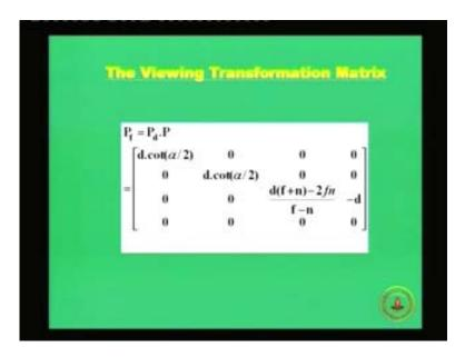
And if you look into the parameters, all the parameters are based on the camera model. If you take d what is the d? d is something you can visualize it to be the focal length of lens, camera parameter where basically the distance of the projection plane from the origin and that is the d. What is the alpha? That is the angle subtended at the vertex of the pyramid.
