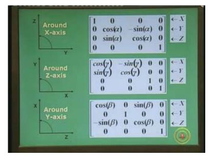
As you can see on the left hand side I have put those three figures, you see the first column, rotation around x axis y to z, rotation around z axis from x to y and rotation around y axis form z to x respectively.
