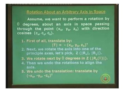
So what do we have here; assume we want to perform a rotation by an unknown theta about an axis in space and now an arbitrary axis because we have seen rotations about three specific coordinate axis x y and z separately, respectively we have seen the forms.
