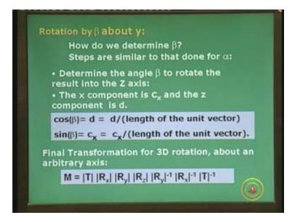
And first is determine the angle beta to rotate the result about the z axis and the x component is  $C_x$  and z component is d. And the cosine of beta is d divided by length of the unit vector is equal to 1, sine beta is this and so beta can be evaluated using cosine beta and sine beta and this gives us the  $R_x$  and  $R_y$  respectively for the second stage. The third stage is  $R_z$  and the last stages are the corresponding inverse matrices.
