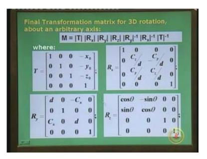
So I write it again, you remember the steps? First translate then corresponding two rotations, then the actual rotation of the theta and then just keep undoing the two rotations about x y and T respectively. Now I must give you the form of all those matrices here T,  $R_x$  and  $R_y$  respectively.
