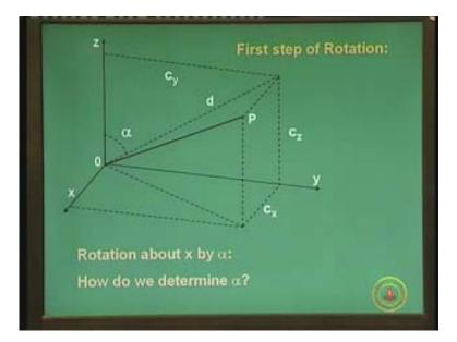
So let us look at the first step of rotation which we said that you need to rotate around the x axis to put it back into the XZ plane. If you remember the previous example, I was saying that you rotate about the x axis to place the axis in the XZ plane. Although it could be the other way round where you can first rotate about y axis and then pickup the x axis but we pickup the x axis first in this case.
