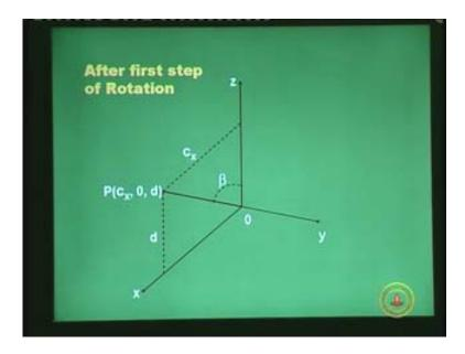
Remember that was our target of step number 2. Step number 2 was to take the axis op and coincide with the z axis. This was the second step of the general rotational matrix and to do that the first step of that second stage of the algorithm is to rotate about x which will give us this particular scenario. So alpha we know now we need to just calculate beta in fact it is done almost in similar manner.
