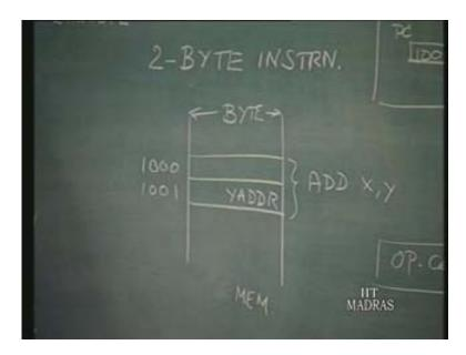
The data fetch is similar to instruction fetch and the address will be placed on the address bus; instead, earlier, PC was pointing to the instruction. So PC confirms that place on the address bus; now the instruction points to Y address and so now, similar to instruction fetch, what it does is Y address is available as part of instruction. Let us note it.
