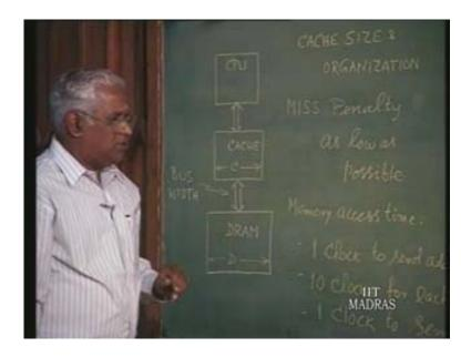
Let us say one clock is needed to send that word to the cache; ten just for accessing and then one more clock is needed to send the data, that is, to send memory word to cache. This must go to cache; only when it reaches the cache, the CPU can access that. So assuming these timings, we will work out. What else do we need to know? You remember what we have been talking about? We are talking about one word block; four word block; multi-word block in general.
