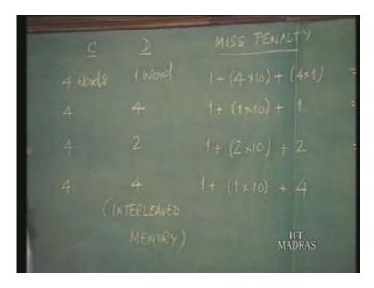
It says, in this case, one DRAM access is going to access four words; so only ten can be accessed at once. Once a reading is to be done, four words will be received, and just in one step, the four will go into the block. So now we have only 12 clocks.
