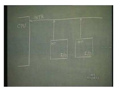
Suppose we have two or three I/O interfaces that is, one for each device, that is good enough. So now the I/O is going to interrupt; the interrupt input is there to the CPU.
