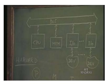
That is the one which has instruction bus and data bus separately and the memory connected to that appropriately: the instruction memory and data memory.
