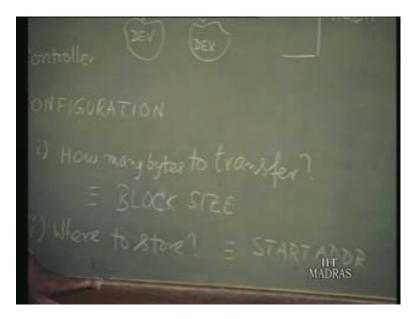
These things must be stored in the DMA controller and that will be done by the CPU during configuration phase. Now we always said I/O consists of configuration phase and data transfer. Since the CPU is not involved in the data transfer, CPU's job is over with the configuration phase because that is all the CPU is involved in. As part of the configuration, the software segment would be something like we will follow the format we followed earlier MOV destination comma source – that is the format.
