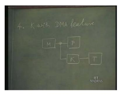
So the processor was involved even in this case whereas in this case, the processor can be removed and the controller can directly access the memory so that between device and memory the data transfer can take place; depending on input output the direction will change. What is the next one? The next one would be this K controller becoming little more sophisticated or complicated with some more complex features.
