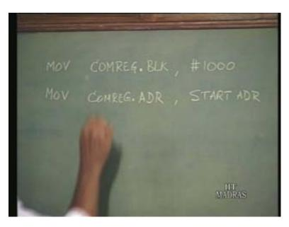
So we will say MOV must go to the DMA controller; I am assuming a command register is there in the DMA. A command register is there and specifically within the command register I may have to move to the part which is going to store the block size.
