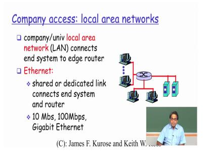
So coming down to a non residential type of network access you typically have a LAN network which we all would have heard of so that is typically based on Ethernet, so when it is Ethernet it is basically a shared or a dedicated link which is connecting the end system and my router device on that particular LAN network so it could be either 10 mbps, 100 mbps gigi and today it is also becoming pretty common to actually have 10 gigabit Ethernet LAN backbones as well.
