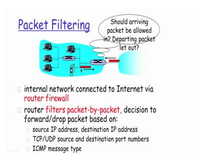
So packet filtering level firewall will basically be filtering the packets on in individual bases right, so I will basically have a different configurations done on my firewall device here, so let us say that I have the firewall device available as part of my network router at my edge itself.
