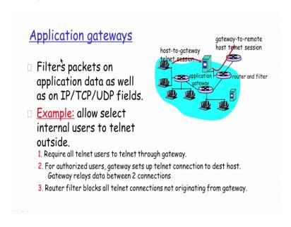
So coming into the application gateway I would basically try to have a application gateway component for each of my applications so all kinds of traffic for that particular application will only be routed through that particular gateway component right.
