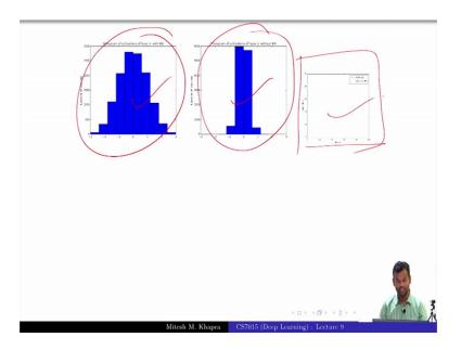
So, here in this figure what I am going to draw is the validation loss, am I no the training loss as I keep increasing the number of epochs and here I am showing you the histogram of the activation functions at layer 1. So, I have trained a deep feed forward neural network and I am showing you what do the activations look like at layer 1 with and without batch normalization. So, remember that we started with this intuition that
