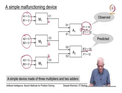
So, what device are we talking about? Here is a standard example, you can find it in almost every textbook on model-based diagnosis and this is a simple malfunctioning device. As you can see there are three multipliers; M 1, M 2 and M 3 on the left. Each of them has got two inputs and they happen to be same in this case 3 and 2, 3 and 2, 3 and 2.
