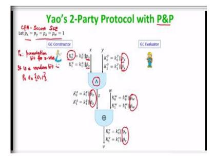
So, let us first see the point and permute technique here. For the purpose of demonstration, I am taking a circuit where we have an AND gate followed by XOR gate which needs to be evaluated. And now we are assuming that we have just a CPA secure symmetric key encryption, which we know how to build using pseudo random functions which can be instantiated using AES. And, we do not require any special correctness property.
