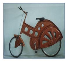
And from these mockup models we built one full scale mockup, non-working mockup because, you know, you need special steels to make a prototype.
