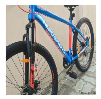
How many of you have ridden aluminium bicycles? Aluminium alloy bicycles? Very good. They are very light right? What happens when the cycle is light? It moves faster with lesser effort right? But the aluminium alloy is so expensive that the cycle generally costs 3 times the regular cycles. 3-4 times the regular bicycles, because aluminium is difficult to weld, and the alloying, you know, is a special process.
