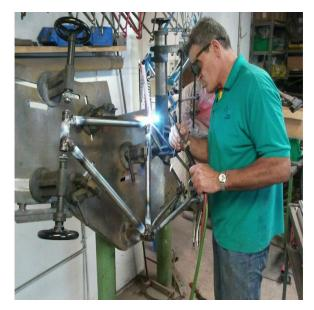
You know, when you weld a frame what happens? When you weld something what happens? When you weld pipes together, the stresses develop in the pipes, right? And your pipes are never in one line. So your front wheel and your back wheel in all our cycles are never true. If they are highly true, they will be the best cycles. You will have a very little load to bicycle. There will be phenomenal. You will see the difference drastically.
