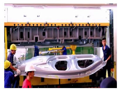
How they were manufacturing cars? They are manufacturing cars by sheet metal draw, right? The car body is drawn by large presses. You may have seen it on videos. So, when the large press is pressed you get the whole part in one go. So, can we manufacture bicycles rather than pipe welding, you manufacture by the deep drawn process.
