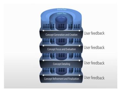
Remember I was talking about the stages in the process. So you have the idea generation here. Then you have the concept focus. You have multiple concepts here, three concepts. You can do the concept detailing, and then you finally do the refinement. So, when you have these stages. You can get inputs from various members very, very effectively into the team.
