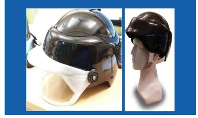
And from the CAD model we did, we did multiple 3D prints, you know, they would be an error over here so we would print again join that. So, in this case is the bottom shell and then we also have the gasket 3D printed. Unfortunately the 3D printed gasket was not very, you know, was not very good. It became very tight when we assembled it. Some other components are very difficult to 3D print because the hard components are very easy. The flexible components are generally it is good to mould them.
