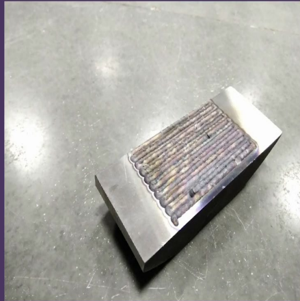
Hard-faced sample of CPM9V on H-13
