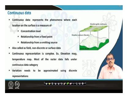
And when you look at continues data I have given I just spoke about the elevation part of it if this is elevation map you can look at the elevation of the grids continuous grids here. So this is nothing but your continuous data, when I represent a phenomena with each location is surface of on a surface is a measure of may be a concentration level, may be relationships okay, may be relationships on a fixed point or from emitting source.
