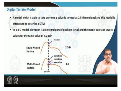
So when you say additional terrain modelled okay the model, which is able to take only one z value, so you can have number of z values at a point of time, but there is if it can only one z value it is termed as a 2.5 dimensional model and is often the called a digital terrain model okay, please understand a model which is able to take only one z value. That is that is what is the crux, one z value its call at 2.5 d model okay
