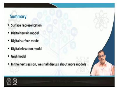
So, this is about the grid model. So when you look at the entire chapter here may be spoke about the surface representation, how do we represent a surface we looked ay that digital terrain model, terrain model, you have a z one z value that defines a digital terrain model, when you have a surface related to it. So you add features on the surface to it then it becomes a digital surface model.
