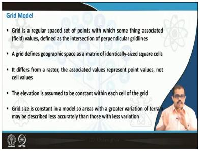
That you should remember that is a basic difference between a DTM and DEM. But in general, both are referring to the same kind of representation. So the next thing as a grid model, grid is a regular space set of points which with which something associated. For example, you have a field values defined as intersection of perpendicular grid lines.
