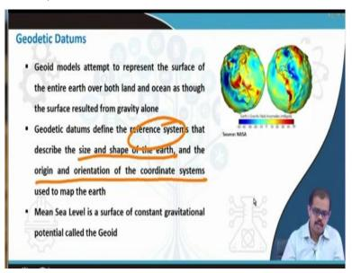
The thing that you have to look at geodetic datums are defining a reference system ok then it describes the size and shape of the what is the size of the earth, the shape of the earth and origin and orientation of the coordinate systems. So all of these together will form a datum ok, so mean sea level is a surface of the constant gravitational pull which I have already spoken about in my previous class ok.
