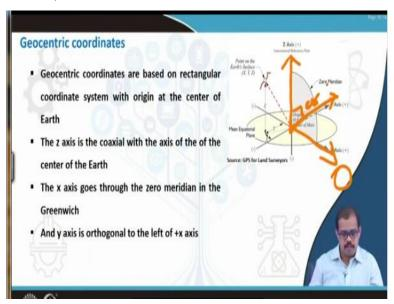
Then next comes a geocentric coordinates, geocentric coordinates was used a in various ways it is extremely important in terms of when you are trying to make the measurements. So geocentric coordinates are based on a rectangular coordinate system with origin at the centre of the earth surface. So if this if we consider this, this is the centre of the earth surface, the z axis is a coaxial with the axis of the centre of the earth.
