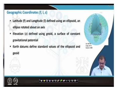
Latitudes and longitude or defined using an ellipsoid or a spheroid and ellipse rotated about an axis ok, elevation is defined using a geoid ok a surface of constant gravitational pull. We have already looked at it an earth datums defined the standard values of the ellipsoid and geoid ok.
