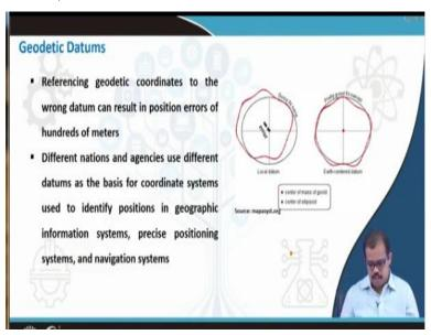
And this is called as a reference grid or a reference point, so when you are looking at a referencing any geodetic coordinates your wrong datum it can actually replicate the position errors to hundreds of meters. So if you are using a wrong datum and you are trying to reference a particular system, then you are if you are measuring it in India, it can even fallen somewhere in Africa, America in terms of where you are placing your map.
