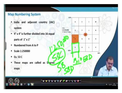
Now let me erase this, this cell this 1degree by 1degree and sorry it is one degree by 1degree right. So now this representation if I say 53D, it is representing this particular map in 1:1 million and the scale of this map is 1:250000 scale, ok. Now we have a 4 degree by 4 degree map ok, that is representing 1:1 million scale divide this 4 degree map into 1 degree by 1 degree map.
