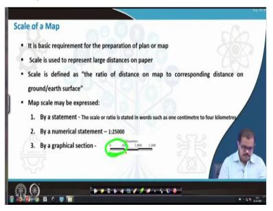
So here when you see this one unit is 500 kilometers on the ground which means 1 unit on the map is equal into 500 kilometers on the ground. So now if we using this unit you can measure what is that particular mid-size, ok, what is the area of that particular image length from one end to the other end etc. can be easily found out with just using the scale that is why you need to, you need a scale for a particular map ok.
