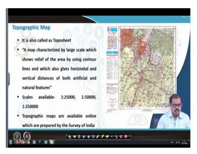
So yeah and when we look at the topographic when I say a topographic map or it is called a toposheet to be more simpler. It is a map that is actually characterized by a large scale which shows the relief of any area by using contours ok and contour lines on which gives you the horizontal and vertical distance of both artificial and natural features that is nothing but your topographic map.
