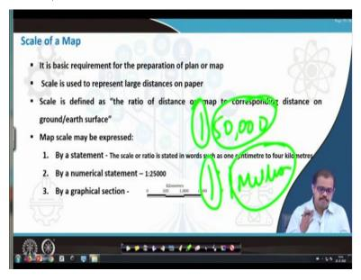
It is a basic requirement for the preparation of plan of a map. So scale is used to represent last distance on the paper, scale is defined as the ratio of distance on a map to corresponding distance on the ground. That I have already said, if I am representing let us say 1:50000 map it mean to say that 1 unit on the map is 50000 units on the ground, ok. If I represent 1:1 million map it means to say that 1 unit on the map is 1 million units on the ground, ok.
