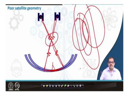
So, you have a poor satellite geometry even in terms of something like this, whether it is joining at a particular position or it is having, so now what happens when it is actually measuring a point, the 2 satellites measure this particular location right. So, now with the previous; the way the previous 2 signals were adding it, it would have given the location somewhere in this region.
