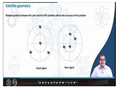
So, when we are looking at this, there is also a concept of how you are relative positioning between the user and GPS satellites are also affected for example, if you have something like this, there is no crisscrossing, so you have a best signal that comes and your measurements is quite precise based on the positioning service you have but if you have something like this, even with a precise positioning service, you may have certain errors induced because of the satellite signals.
