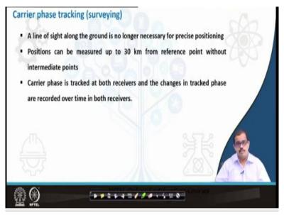
So, when you are looking at this, the first thing that application that you can see is; surveying, the carrier phase tracking. So, when you look at it a line of sight along the ground is not necessarily a precise positioning, okay. If you have any line of sight across your entire surface, then it may not be your precise positioning. Positions can be measured up to 30 kilometers from the reference point without intermediate points, please keep this in mind.
