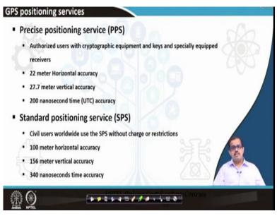
So, when we look at GPS positioning system, we have 2 types; one is the precise, another one is a standard and standard, when we look standard is for most of the countries which actually is a list of positioning system where the accuracy is very limited and when you look at
