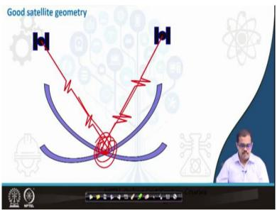
To give an example of signal error, so this is; this is what it means so, you have a satellite signal that is reaching and this is a satellite and that was crisscrossing each other because of which the error is actually induced into the system, okay.
