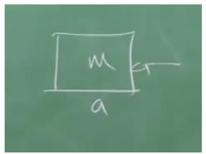
There are simple models, the simplest model you can think of is just vehicle consisting of mass m okay one mass, the vehicle as an acceleration a okay and has a force opposing its motion so a becomes deceleration, will call that s, a we will not call acceleration deceleration every time we just call that depending about positive or negative you can come to your own conclusion.
