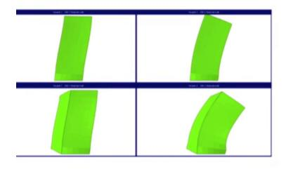
So I can do 2 things, one is that both of the bottom and the top are fixed not to move in the z direction okay both of them are a guy stuck between 2 plates this is what happens to a block when it is in the middle of the contact patch, at the edges of the contact patch one guy is free okay, so I can free him I can free him okay we will apply this load, let us say that I have a square cross section I applied this load okay what do you expect?
