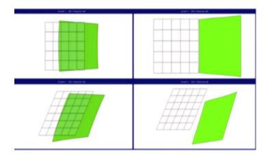
Now that is the top view see what has happened let us concentrate on the left side, so left side clearly shows that this is a finite element picture is just an isotropic rubber block, so it shows that when I apply a force F the displacement Fx let me call that as Fx, the displacement is only in the x direction for that rhombus okay which is very similar to that there in the tread block, if I apply a force Fx.
