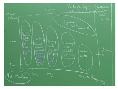
So the vehicle oscillations can be classified in terms of frequency of oscillations okay, and the amplitude of oscillations, right. So, yes when you when you talk about oscillations immediately you think that there is going to be a bounce when a vehicle goes over a rough road and you see that there is no bounce and so on and immediately you have a tendency to sort of map this word oscillation to a vertical oscillation right.
