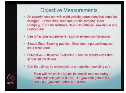
We also said that the experimental car which Chen and Ash used at the Leeds University, they had 8 vehicle parameters, okay and then these 8 vehicle parameters were changed and 16 configurations were arrived at or 16 different cars were the ones which were tested. Of course, Adams model is being used as well in order to get the objective rating and experiments were conducted in order to obtain these ratings as well, okay. So let us now look at what are the type of questions.
