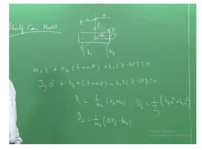
And then we moved over to what is called as the half car model, right? So in half car model, we said that we will take a very simple case, we have say for example, we are going to remove, in fact the unsprung mass. We will consider only the sprung mass and that the sprung mass along with the moment of inertia perpendicular that is J theta form the 2 constants of the car, of the vehicle.
