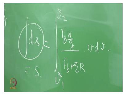
So, in other words, what I am going to simply do is to take this to the right-hand side, rearrange it and write it as gamma Bw/g/Fb+sigma R\*vdv and then integrate the left-hand side and the right-hand side, okay. It can be from say v1 to v2 and the corresponding distance we would call when it comes from velocity v1 to v2, we will call it as yes, so that this would become yes. As I told you there is small twist.
