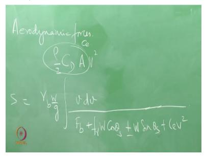
What is the twist, the twist is because the resistance here involves aerodynamics forces. Aerodynamic forces can be written by rho/2 dense to the air, very important co-efficient drag coefficient CD multiplied by the projected area A\*v squared. So, since v squared is there, I cannot take that out of the integral, so I have to re-write that integral S to be equal to, I can take
