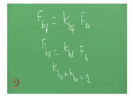
We also said we went to the next step and we said that we can dump the whole of the effect of tyre on to the road, then the whole concept of this interaction into a factor called mu which is very similar to your well-known friction condition, the Coulomb's friction and said that W\*mu will give me a limiting condition for the wheel to lock. So, in other words, the maximum force that it would take front or rear would be given by this condition.
