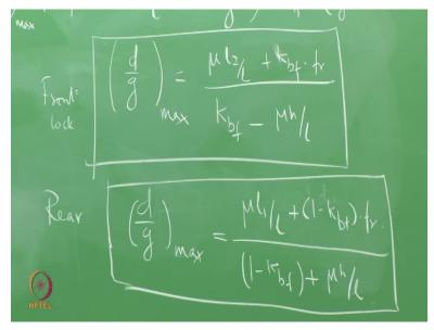
Derive the expression for, when is this condition, this is front wheel locks, okay. The maximum deceleration that is possible when the front wheel locks, okay. Now, derive what should this be when the rear wheel locks. What is the condition, just put this, substitute it, and rearrange it. See that you get this, this would be the condition. The same thing, I have 2 versions of the same equation. I am equating it, rearranging the terms, and I am getting this, okay.
