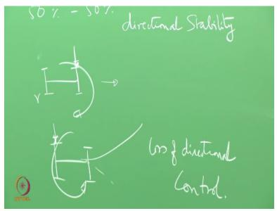
Let us say that I have a vehicle, just to schematic diagram of vehicle, okay which is traveling in this direction, of course and let us say that one of the wheels locked. Let us say that rear wheel is locked. What is meant by locking physically or from a physical principle. Locking simple means that all the mu that is available for that tyre has been completely consumed, right. So, no more that mu factor, the friction factor is available for any other force that axe the wheel, right.
