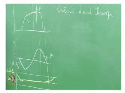
That some of this area under this contact patch, contact pressure multiplied by that is in other words, if I say that the contact pressure is P okay which is a function of x, y dx dy, if I integrate the whole thing okay is the total reaction of the ground okay that we are talking about, all right. As we had seen earlier, this is not symmetric for a rolling tire with the result that, there is an unsymmetric distribution results in a force that acts, which is responsible for rolling resistance.
