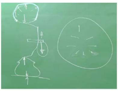
And there is a spokes which has an initial tension, it is a ground, so the equilibrium demands that the whole wheel hangs it, hangs the axle from the top. This is exactly what happens in a tire but who plays the role of the spokes in a tire, it is the sidewall of the tire. So, let us draw the sidewall okay, let us say that that is the sidewall of the tire okay, they are; say let us say sitting in a rim, all of you have seen a rim, okay.
