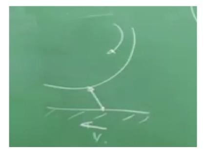
It is very important this; very important to understand that the tread elements can be extended or can be; or extended in either direction, I would say, okay extended in either direction. Just to under; before I go here; let us understand this carefully. Let us say that, that is the wheel okay and let us say that there is a tread element which is sitting that is the carcass rather okay, the treads are blocks which are extending from the carcass body of the tire, right they are extending.
