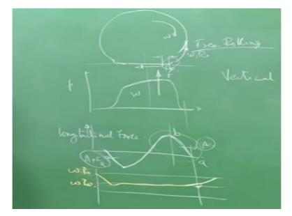
So, when I extend that concept to free rolling, this is free rolling and assume that the friction is good enough that there is no slip okay; here slip what we mean is slipping of this? When the force; say there is a tangential force; the tangential force is higher than the; what can be withstood by the frictional force then it would start slipping okay. We will come back to that figure again; we will be talking about that figure more often now.
