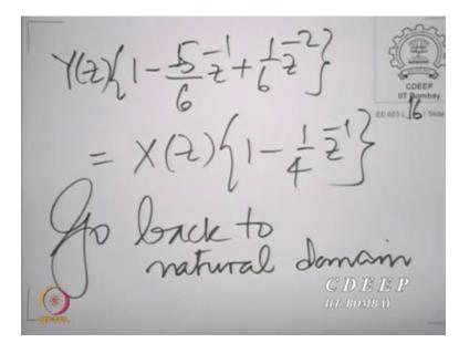
We can cross multiply to get Y Z into 1 minus 5 by 6 Z inverse plus 1 by 6 Z raise to the power of minus 2 is X Z into 1 minus one fourth Z inverse. And we can go back to time, go back to the natural domain, by taking the inverse Z transform both sides. So of course, it is very easy to see that you would get y n here and here, you would get minus 5 by 6 the inverse Z transforms Z inverse Y Z is Y of n minus 1, eventually y delayed 1 and so on
