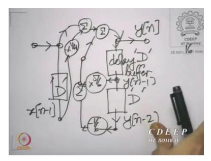
So, in fact, suppose you happen to have, you know, a circuit which constantly generates y n, that means you have, you know let us assume that you have a timing mechanism, which times the samples, the sampling points and the samples. You know, in every in every unit time, one sample of the input is fed, and one sample of the output is generated. So, you have a timing mechanism, you have to have a timing mechanism.
