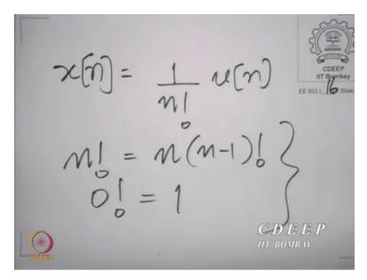
In fact, it turns out that this sequence x n would simply be 1 by n factorial u n, where n factorial has been defined already and u n, u n is the unit step. In fact, very interestingly, if an LSI system were to have this impulse response, suppose, x n where the impulse response of an LSI system, we could ask whether the system is causal and stable.
