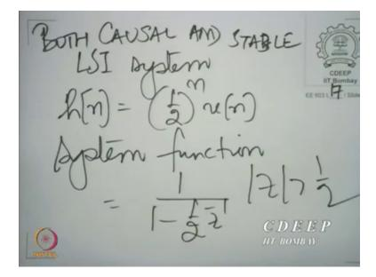
So, if you have the system, LSI system with impulse response h half raise to the power of n u n, the system function is 1 by 1 minus half Z inverse mod Z greater than half. And this is both causal and stable. So, now we have an example of all 4. In fact, we will take this example or this pair of examples to draw some conclusions.
