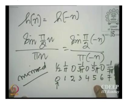
And let us therefore write down the impulse response for a few values. In fact, we can again simplify it, you see h n is equal to h minus n. It is an even impulse response, that is very easy to see. That is because sine pi by 2 n by pi n is equal to sin pi by 2 into minus n by pi minus n, that is very easy to see. And therefore, we can write down the impulse response only for a few values say 0 to 10 as I said 0, 1, 2, 3, 4, 5, 6, 7, 8, you can go on.
