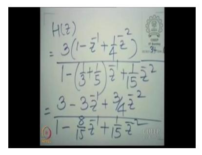
And therefore we need to expand this, let us do so. So  $H(z) = \frac{3(1-z^{-1}+\frac{1}{4}z^{-2})}{1-(\frac{1}{3}+\frac{1}{5})z^{-1}+\frac{1}{15}z^{-2}}$ . So that can be
