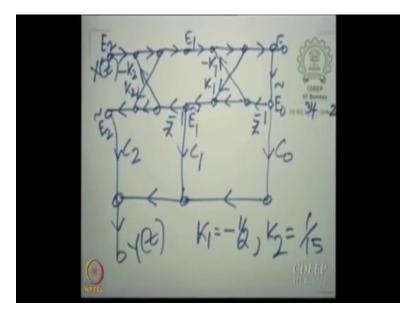
And as expected the denominator polynomial yields both lattice coefficients less than 1 in magnitude as was the necessary and sufficient condition. This is a verification; not a proof, but a verification. Now we need to determine the  $c_0$ ,  $c_1$ ,  $c_2$ . So let us begin. Now we know what these are, we know what the A's are.
