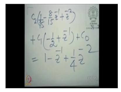
$c_2 \widetilde{A}_2(z)$  which is  $c_2 \left(\frac{1}{15} - \frac{8}{15}z^{-1} + z^{-2}\right) + c_1 \left(-\frac{1}{2} + z^{-1}\right) + c_0 = 1 - z^{-1} + \frac{1}{4}z^{-2}$ . As expected the coefficient of  $z^{-2}$  can be compared on both sides; it comes only from here.
