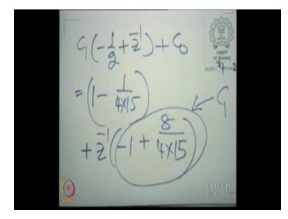
So, therefore  $c_1\left(-\frac{1}{2}+z^{-1}\right)+c_0=\left(1-\frac{1}{4\times 15}\right)+z^{-1}\left(-1+\frac{8}{4\times 15}\right)$  and the  $z^{-2}$  term is annihilated. And therefore  $c_1$  is now very clear as well. This is essentially  $c_1$  now. The coefficient of  $z^{-1}$  is  $c_1$ . So once you have  $c_1$  you can subtract this term from this side again and find  $c_0$  finally. We can continue this.
