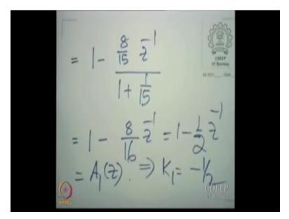
And therefore the coefficient of the highest power of z namely  $z^{-1}$  in  $A_1(z)$  is essentially  $K_1$ which means  $K_1 = -\frac{1}{2}$ . And once you have  $K_1$  you have completed the lattice for the denominator. But now we need to write the lattice for the numerator. Essentially what we have is a lattice of the following form. We have an  $E_2$  there.
