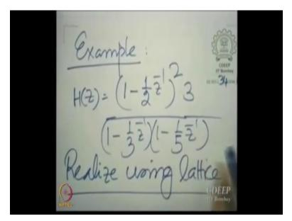
The system function has poles which are both inside the unit circle and therefore the system is stable.
