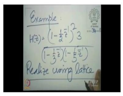
Let us construct  $H(z) = \frac{3(1-\frac{1}{2}z^{-1})^2}{(1-\frac{1}{3}z^{-1})(1-\frac{1}{5}z^{-1})}$  if you like using the lattice structure. Let us expand
