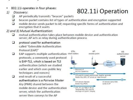
These phases are illustrated in this picture. Again, this is the mobile device, this is the access point, and this is the authentication server. And these phases are as follows. The first phase is the discovery phase, in which the mobile device discovers the security mechanisms that are available with this access point. The access point periodically transmits beacon packets.
