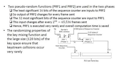
So, hence the input to PRF1 changes after every 2<sup>16</sup> frames sent. Hence, PRF1 is executed very rarely, and overall computation time is saved. So, every frame only PRF2 has to be executed, and PRF1 is executed once every 2<sup>16</sup> frames. So, that saves on computation cost. And the randomizing properties of the key mixing function and the large size, which is 128 bits, of the key space ensure that key stream collisions occur very rarely.
