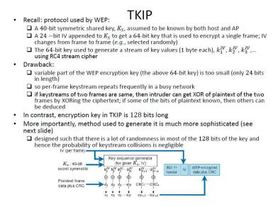
It was assumed to be known by the host as well as the access point. So, that is this key, K<sub>S</sub>. It's a 40-bit secret symmetric key. And a 24-bit initialization vector was appended to this key K<sub>S</sub>. That resulted in a 64-bit key, and this 64-bit key shown by these two arrows here, this is used to encrypt a single frame.
