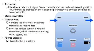
The next component is a microcontroller, which receives the information collected by the sensor and sends commands to the actuator to take different actions. It also is connected to the memory, and so where data is stored and programming data are stored in the memory. Another component is the transceiver. That is shown here. It contains the electronics required to transmit and receive data.
