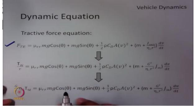
so we know the force equation as addition of different forces. And let us now substitute you know torque of the vehicle axle on FTE, so we know FTE is torque of the wheel divided by R and also the relation of J axle with respect to inertia of the motor.
