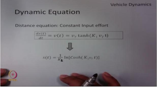
We can also use this equation to find the distance the system travels in a finite amount of time, so VT is nothing but D/DT of ST, so S is basically distance, so if you integrate this we can get the expression of S(T), so S(T) is 1/K1 logarithmic of cos H K1 VT, so this is exponential graph and let's say we want to understand you know the starting acceleration, (Refer Slide Time: 31:45)
