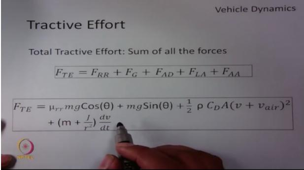
So we have seen that the total effort that is required to move the vehicles you say sum of various forces such as force due to rolling resistance, force due to gradient or slope, force due to aerodynamic drag, and force that is required such as linear acceleration and angular acceleration, if you want to provide change in a speed when the vehicle is moving.
