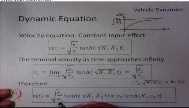
So this infers at this the velocity will start from let's say 0 meter per second and it will move towards statistics value as that time elapses, so what is the statistics value of this velocity?
