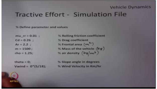
so the simulation file use to plot this graphs is elaborated here, so first general in the summation file we have to define the parameters and their values, so in our case we need to define the rolling friction coefficient which let's say Mu RR, it's a 0.01.
