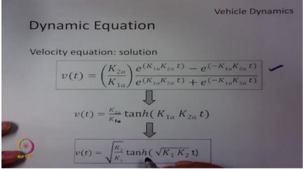
can be easily rewritten as V(T) is K2A/K1A Tan H (K1A, K2A into T) so this is the equation we were looking at, so this can be further simplified and we will again re-substitute the value of K1A and K2A in terms of K1 K2, so K1A is route of K1 and K2A is route of K2, so if we substitute this we'll get this equation.
