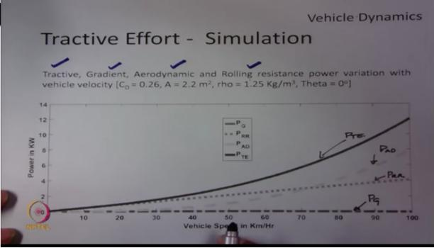
Now let us see all the forces and their variation together, so let us see the gradient force, the aerodynamic force and rolling resistance force and addition of this force is which is attractive effort together in a same graph, so we want to see the effect of this vehicle velocity on this forces and the power variation.
