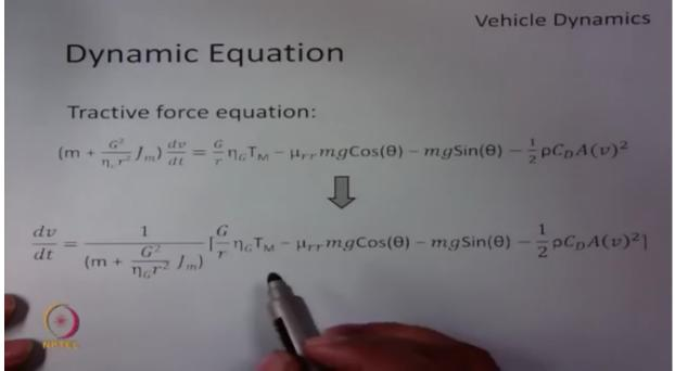
so if we re-substitute the thing and we bring this term which is proportional to DV/DT on one side, and the tractive effort and the subtraction of all the resistive forces on other side we can get this equation D/DT will be G/R eta G TM – all the resistive forces and this will be divided by the equivalent mass on the vehicle axle.
