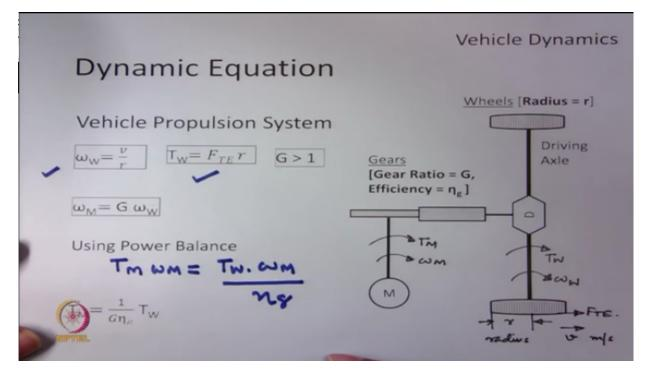
So since we know the relation between omega M and omega wheel we can find the relation between TM and T wheels as this, so TM will be 1/G eta G into T omega, so here we can see that the motor torque is lower compared to wheel torque since it is divided by G and G is greater than 1.
