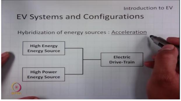
During acceleration we want the system to be fully utilized therefore during acceleration both the system will deliver power or energy to the drivetrain such that the system operates at very high power rate,
