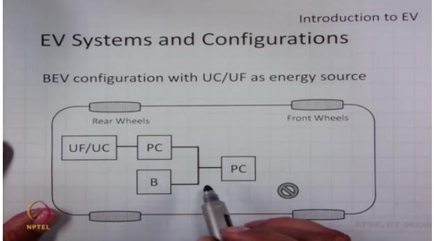
this devices have high specific power and it can very well support the high specific energy of batteries, so this are generally a low voltage devices and it generally requires a boost converter which has to be bidirectional because this can be recharged quickly when the power is coming back from regenerative braking.
