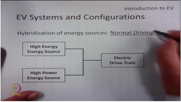
so in case of normal driving the high energy source is mainly used to drive the vehicle such that we obtain a high range operation, independently the energy flow can also happen from high energy source to high power source when we have a light load or very low power requirements in a drivetrain, so this is normally to transfer energy from high energy source to high power source, so high power source generally cannot store energy on its own.
