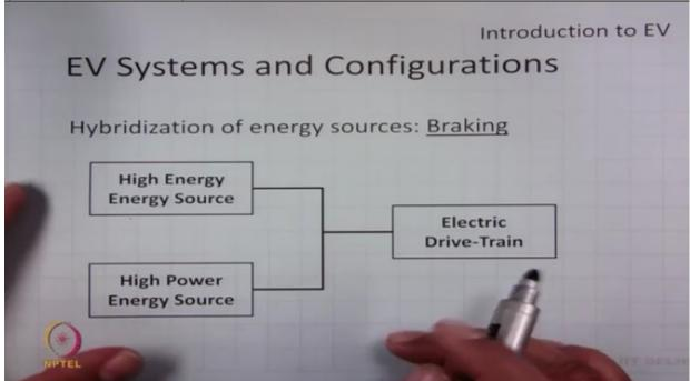
so during braking the energy has to be observed very quickly, so during that time the main source which recovers the braking energy is high power source, since it's a capacity to observe power very quickly, but this can also be used to recover the energy but this is preferred because it can support very quick recovery of braking energy, so this is first priority and this is second priority.
