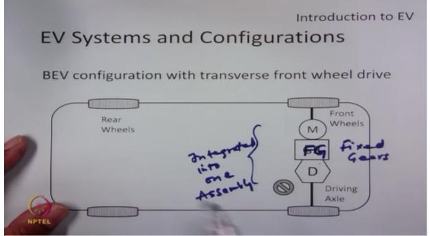
so this is adopted in all modern EV's, even this kind of technology is used in tesla vehicles, so we all know that differential is a very important mechanical device which is used to create (Refer Slide Time: 18:47)
