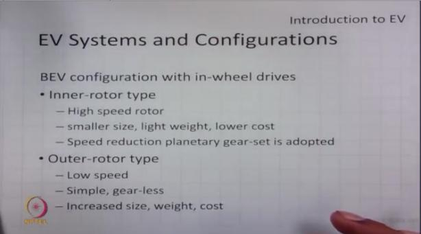
So if you see these two systems the first type of in-wheels system is in a rotor type, means it can be a conventional motor with a high speed rotor, and the speed reduction is obtained by a
