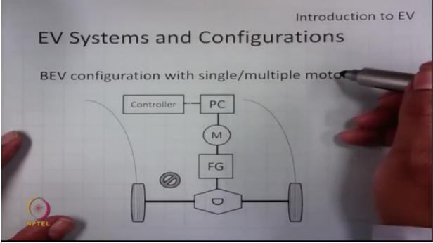
so let us see what is the difference between a single motor or a multiple motor based BEV configurations, so we all know that when we use a single motor we have to use a differential, so what is this differential? Differential is basically a third gear system like, so one gear which is called pinion gear and connected to two axle gears, so depending upon the requirement of turning the vehicle can be turned.
