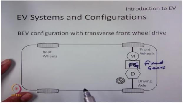
all the components such as motor, fixed gears and differential are integrated together, so these are all integrated into one assembly such that the transmission axle is reduced and it's a very compact system such that it not only takes the very less value, it is very less weight compared to the previous configuration,
