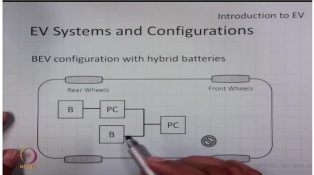
therefore normally we go for hybrid battery systems, so in hybrid battery systems two batteries are used to operate the motor and this battery will be connected using a power converter such that the power flow between this batteries can be controlled.
