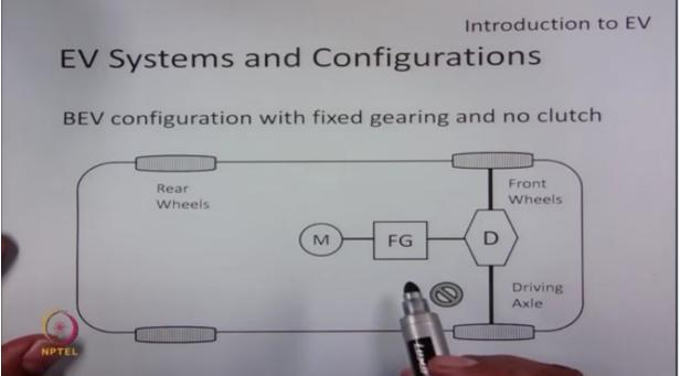
so this system uses electrical motor with a fixed gearing, so here your fixed gear ratio typically 1 is to 10 ratio is normally used.
