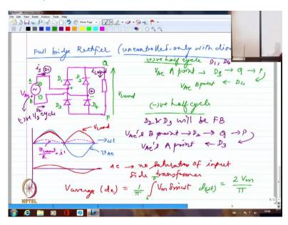
So, we are going to call this as uncontrolled bridge rectifier which is only with diodes, so we call this as uncontrolled. So, I normally draw it like this, I am sure you would have learnt it sometimes differently with diamond kind of structure and so on but it does not matter because this is easier for us, especially when we are going to go to three-phase rectifier. So, I would like to draw it somewhat like this with the load here and power supply at this point.
