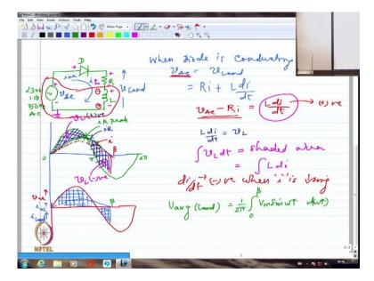
And I am going to have a sinusoidal voltage here. Now, again I am going to have 230 volts single phase 50 hertz AC. And I am assuming again ideal diode, no doubt. So, when the diode is conducting and I am assuming that the diode is not having any forward voltage drop or negligible voltage drop, so I should say when diode is conducting, I am going to have  $V_{AC} = V_{load}$ , if I say this is what is  $V_{load}$ , I should say  $V_{AC} = V_{load}$ .
