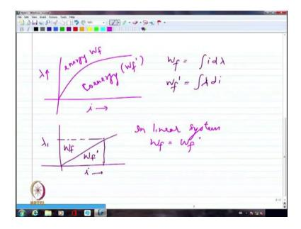
And we said if we are actually plotting a graph between i and  $\lambda$ , we are probably going to plot it like this with non-linear characteristics. If I say that there is an iron core which is contributing to non-linearity between the relationship between i and  $\lambda$  or N $\phi$ .
