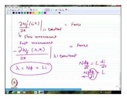
So, let me write these two expressions once again. Let me write that  $\frac{\partial W_f'(i,x)}{\partial x}|_{i = \text{constant}} = \text{Force}$ . This is for slow movement. If I consider fast movement under that condition, I am going to have  $-\frac{\partial W_f(\lambda, x)}{\partial x}|_{\lambda = \text{constant}} = \text{Force}$ .
