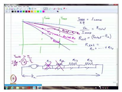
So, I can design rather a starter such that I would probably have the minimum and maximum values of torque pre-decided maybe I know what is the kind of load that is coming up on my DC motor. So, for which I have to make sure that the maximum torque that is actually generated maybe, twice or three times whatever is the load torque, so that enough acceleration comes. So, what I need to do is maybe fix up two limits, one will be  $T_{\text{max}}$  one will be  $T_{\text{min}}$ .
