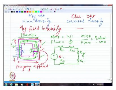
And we also said when we were talking about flux density in the case of a magnetic circuit that is corresponding to current density in the case of an electrical circuit. If I am looking at magnetic field intensity whereas here, there is no corresponding quantity, although one of your classmates mentioned that electric field is V/m, so we should be able to say that as an equivalent quantity, invariably, we talk about electric field only in electrostatics.
