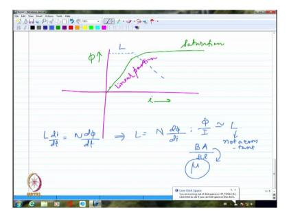
If you actually plot this, you are going to have it somewhat like this, let us say this is the x-axis and this is the y-axis. So I am going to have essentially on the x-axis, I am going to have I and on the y-axis, I am going to have the flux. So initially, I may say that as I increase the current, the flux is increasingly linearly, but beyond a particular point, the increase will become you know less and less and it will become almost flat.
