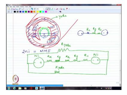
If I take a DC machine, there will always be a stator and there will be a rotor. The stator in the case of DC machine produces the magnetism that is required which is acting like a via media between electromechanical energy conversion process. So let us say this is going to be my stator's outer periphery. So I am going to have basically a magnet here, I am showing it like this and one more magnet here.
