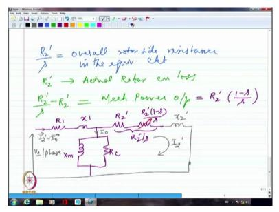
So, I am going to have basically, here I am going to divide this into 2 portions one is going be  $R_2$ ' which is the inherent resistance of the rotor circuit converted into the primary side this I
