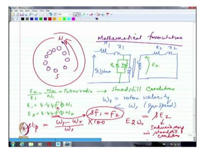
So, in a 2 pole machine, it is going to continuously rotate, and I have the rotor conductors sitting here, these are the rotor conductors, the rotor conductors are looking at this particular revolving magnetic field, it is definitely seeing a rate of change. So, there will be an induced EMF.
