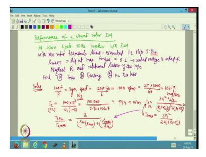
Let me work out 1 more problems on the performance of a wound rotor induction motor. The problem statement goes as follows it is a 3 phase, 420 volts, 6 pole, 50 hertz, 100 kilo watt wound rotor induction motor. What is written is with the rotor terminals short circuited we are going to have the full load slip to be 0.04 and slip at maximum torque that is  $s_{max T}$  is given to be 0.2 when it is running at rated voltage and rated frequency.
