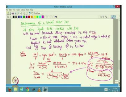
Now, using this we should be able to write  $\frac{T_{eFL}}{T_{emax}} = \frac{2}{(\frac{0.04}{0.2}) + (\frac{0.2}{0.04})}$ . All these things are known
