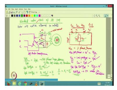
We had seen the open circuit test of the induction motor. We have to look for the next one which is known as blocked rotor test of 3 phase induction motor. So, as the name indicates in this particular case rotor will be blocked or it will not be allowed to rotate. We are going to have the rotor completely blocked. So, when the rotor is blocked we are essentially looking at let me first draw the diagram corresponding to this.
