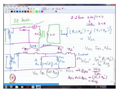
So, let us look at now the short circuit test calculations. So, I am going to have  $V_{sc}$ ,  $I_{sc}$  and  $W_{sc}$ .  $W_{sc}$  will give me only the real power quantity, which will be very clearly  $I_{sc}^{2}(R_{1}+R_{2})$ . Only two resistances are there and only they can dissipate real power. So, what I get actually as  $W_{SC}$  will be  $I_{SC}^{2}(R_{1}+R_{2})$ , and from here I should be able to get what is the value of  $R_{1}$  and  $R_{2}$ .
