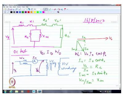
So, let us start off with what we had left off in the last class, BH loop, yes. So, we were looking at open circuit test and short-circuit test. If you may recall, we had drawn the equivalent circuit, overall equivalent circuit of the transformer, we also drew the phasor diagram. We said this is  $R_c$ , this is  $X_m$  and here is  $V_1$ , what we are applying. So, now this is  $R_2'$ , this is  $X_2'$  and then this is what is our load, which we are calling as  $Z_L'$ .
