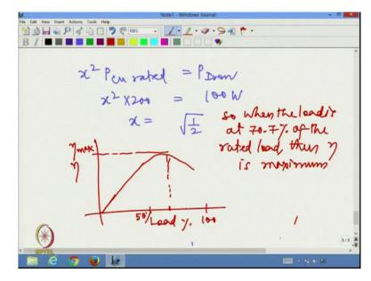
So, I can write this as  $x^2 P_{\text{curated}} = P_{\text{Iron}}$ , so this is  $x^2 200 = 100$  W, so  $x = \sqrt{\frac{1}{2}}$ , so when the load is at 70.7 percent of the rated load, then efficiency,  $\eta$  is maximum for this particular transformer. So, if I try to plot actually efficiency versus load condition, so let us say this is
