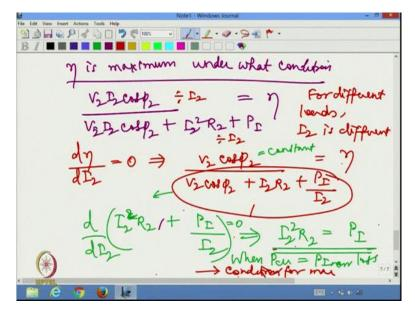
Now let me write, under what condition efficiency is maximum, let me try to derive this under what condition, So let me write the expression  $\frac{V_2I_2\cos\phi_2}{V_2I_2\cos\phi_2+I_2^2R_2+P_1}$ , this is the efficiency, so let me write under different load condition, I am going to have I<sub>2</sub> to be different, so let me differentiate the efficiency with respect to I<sub>2</sub> and I make it as 0.
